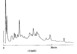
**Figure-13 Separation of urease (Jack Beans)** Conditions are identical to Figure-12. However, sample: 10 g/L, 100 μL
