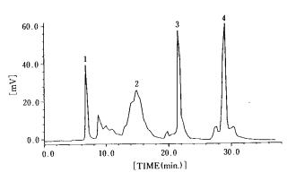
Figure-2Separation of protein mixtureConditions are similar to Figure-1.However, sample:1. Carbonic anhydrase (2mg)2. Transferrin (4mg)3. Ovalbumin (5mg)4. Trypsin inhibitor (5mg)Injection volume 100μL
