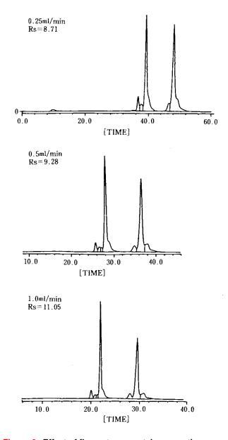
Figure-6Effect of flow rate on protein separationColumn:TSKgel SuperQ-5PW 7.5 mm ID × 7.5 cm LConditions are identical to Figure-1.However, Flow rate: 0.25, 0.5, and 1.0 mL/min.
